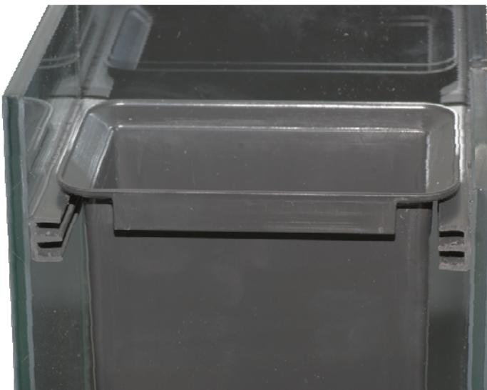
The filter basket can be hung up from above into the retaining profile (as shown in the picture). In this way, it can be removed at any time. The rear wall does not have to be removed. If the basket is inserted into the upper rail of the profile when the rear wall is pulled out, only one filter bag can be removed without removing the rear wall.
