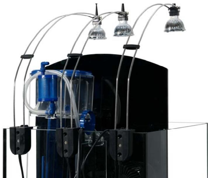
Afterwards, each light has to be put in the corresponding holding unit. The shorter light has to be put into the middle. The light power lines have to be connected to the transformer.
